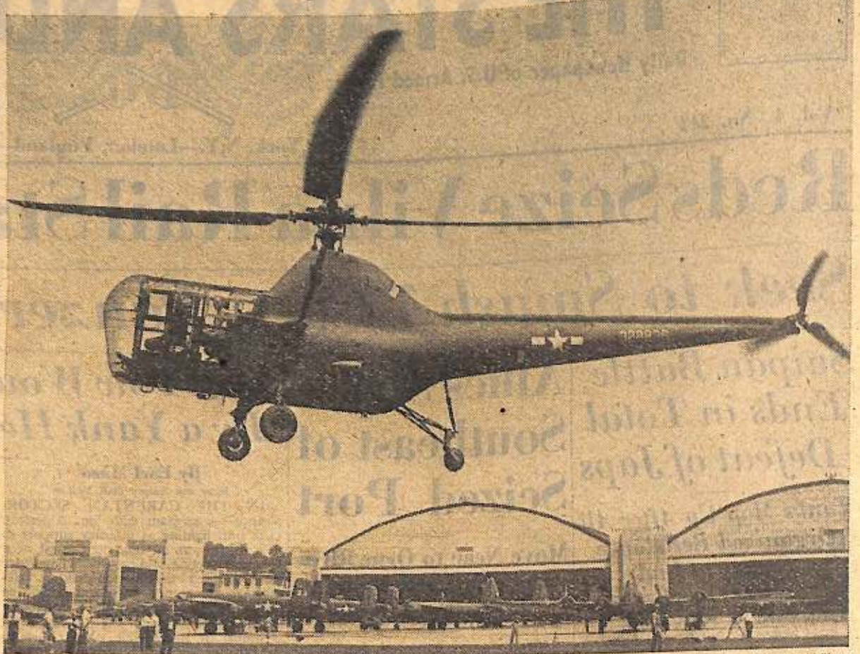
Here is the Army's new XR5 helicopter, built by the Sikorsky Co. It can take off and land vertically, has a speed of more than 120 miles an hour and can carry more than 1,100 pounds, including pilot and observer
