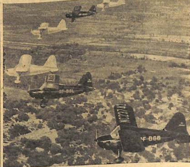
Many of the "Flying Minute Men" flew Stinsons such as these in the patrol flights along the coasts searching for subs following Pearl Harbor. These Stinsons are two-seaters, and fitted with bomb racks and have a top speed of 110 miles an hour.
