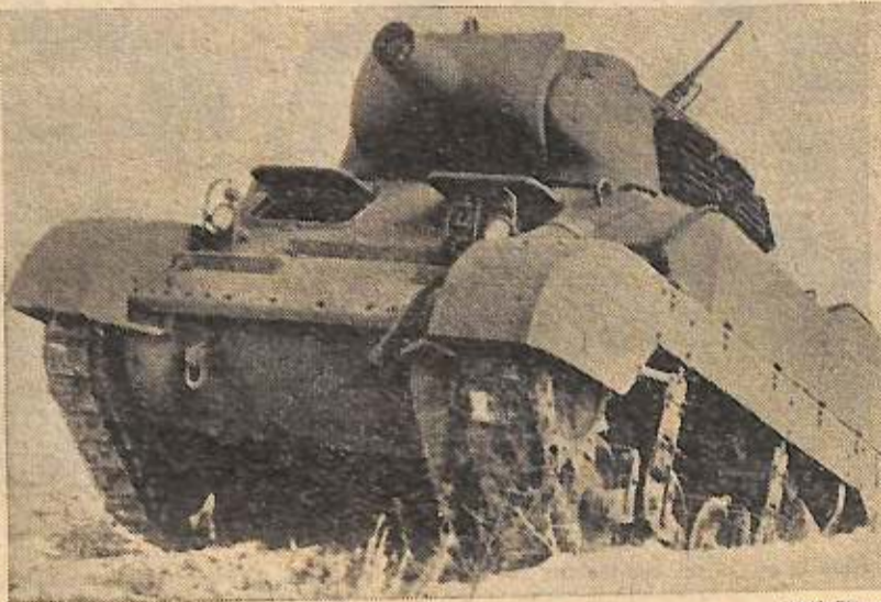
This is the Army's new M8, a light tank mounting a 75mm. howitzer and a .50 caliber machine-gun. Military officials have disclosed that the M8 is being used to form a combat team with M5 tanks, lobbing its mortar-type shells into concealed enemy positions that can't be reached by the low trajectory fire of the M5. This scene was taken during recent tests in the States.
